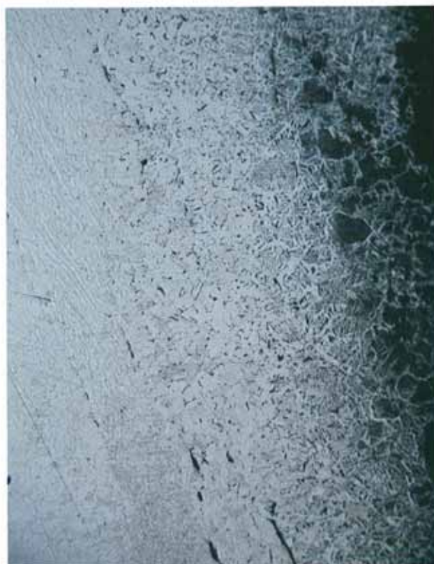
Fig. 13: Demirköy the back-scattered electron image of the consolidated bloom forged in a blacksmith shop.
